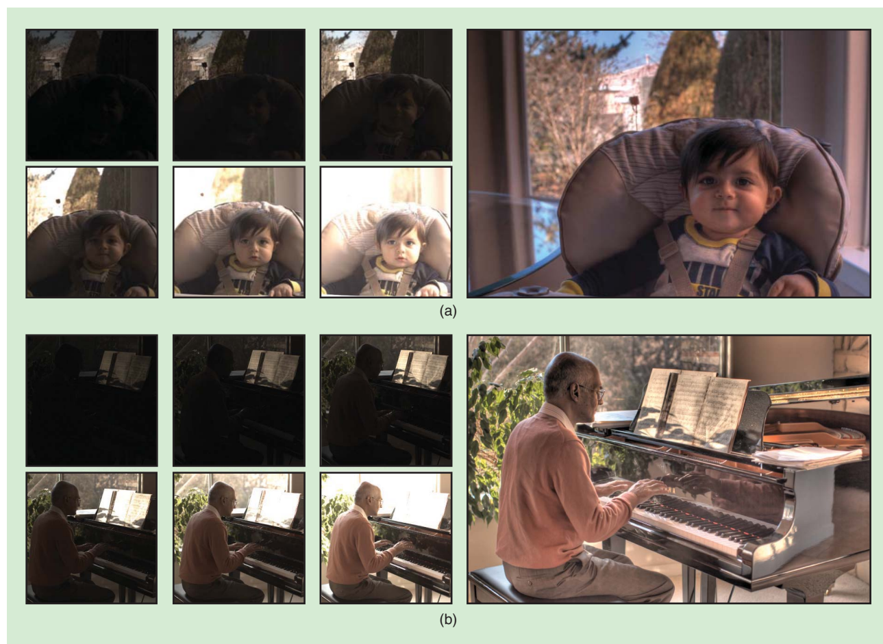
FIGURE 6. (a) and (b) show sample HDR results (right) from the input LDR images (left) using the patch-based optimization of Sen et al. [1].
