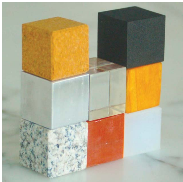
FIGURE 5. Cubes of different material composition (cork, foam, aluminum, acrylic, maple wood, granite, bakelite resin, and silicone); Architect's Cubes Museum of Modern Art, New York. (Photo courtesy of Kristin J. Dana.)
