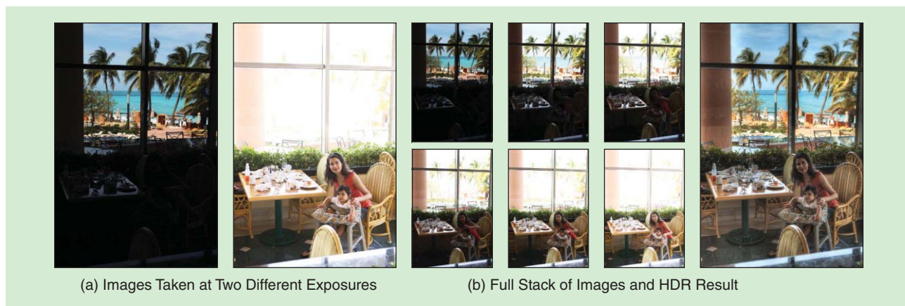
FIGURE 1. (a) Images captured by standard digital cameras cannot reproduce the wide range of illumination we see in everyday scenes, even after adjusting the exposure, as illustrated by these two images taken at different exposures. (b) HDR imaging allows for the capture of a wider range of illumination; here, a stack of images was captured at different exposures (left) and merged with the algorithm described in [1] to reduce motion artifacts and produce the result shown on the right.
