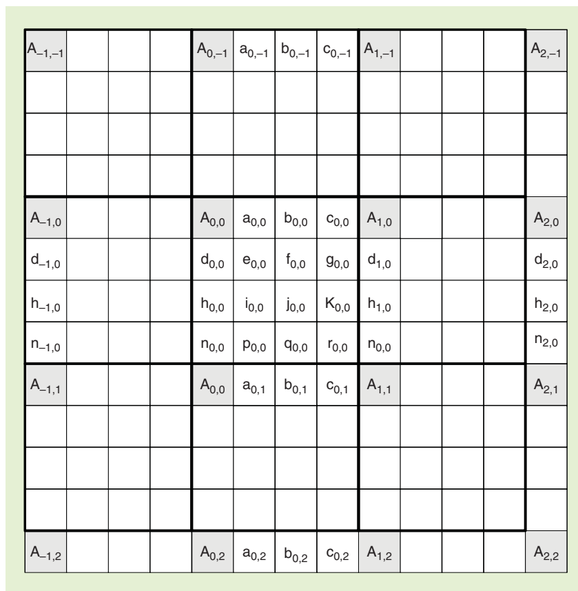
FIGURE 6. Integer samples (shaded blocks) and fractional sample positions (unshaded blocks) for luma interpolation.
