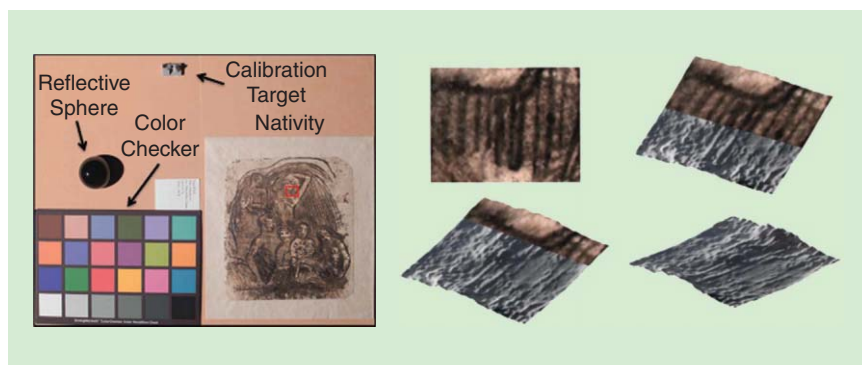
FIGURE 2. (a) The setup for capturing photometric stereo of Gauguin's Nativity : a color checker for color calibration, a 3-D calibration target for 3-D surface calibration, a reflective sphere for calibrating light direction, and the work of art. (b) Several frames from an animation visualizing the 3-D surface shape at the location of the lines drawn in Nativity . The 3-D reconstruction shows clear evidence of protrusions on the page where ink has been deposited. This is solid evidence for the ink being transferred from a matrix such as that in a monotype transfer process. (Images and figure caption used with permission from [9].)
