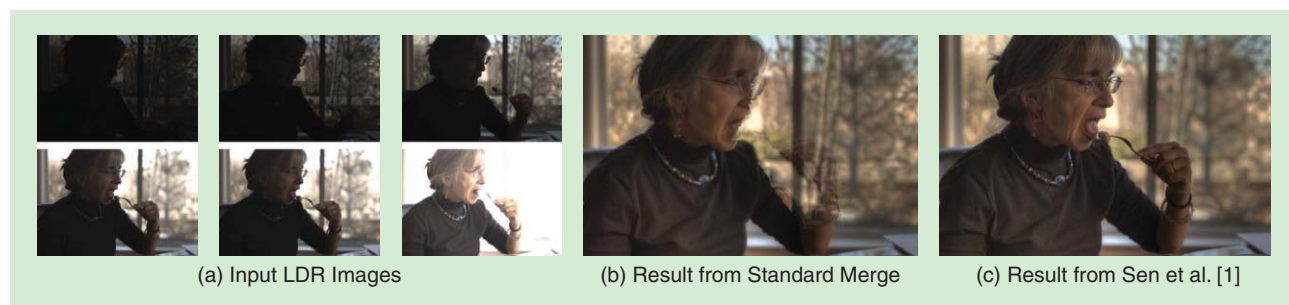
FIGURE 5. Ghosting artifacts can occur when stack-based HDR algorithms are applied to dynamic scenes. (a) Stack of input LDR images. Note, how some images capture the details in the dark sweater, while others capture the detail in the bright exterior. (b) HDR results from the standard HDR merging algorithm produces ghosting artifacts because of the motion. (c) HDR results from the patch-based optimization algorithm of Sen et al. [1] contains detail in all regions of the image without artifacts.
