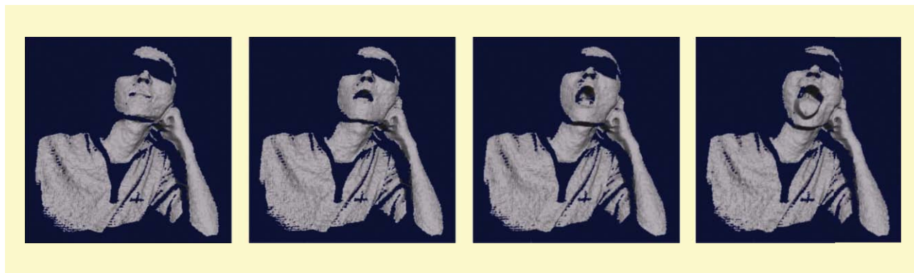
FIGURE 4. Online 3-D reconstruction results of a dynamic scene (facial expressions with black eyeglasses) using three speckle-embedded fringe patterns.
