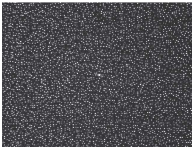
FIGURE 1. An infrared camera image of part of the speckle pattern projected by the Kinect.
