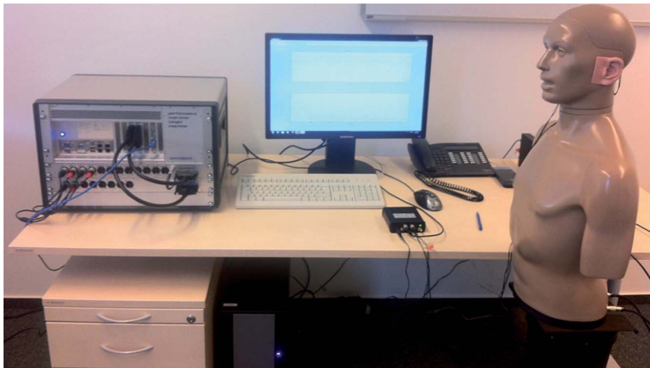
FIGURE 8. The real-time Speedgoat system (left) and KEMAR (right) at the Audio Processing Lab.
