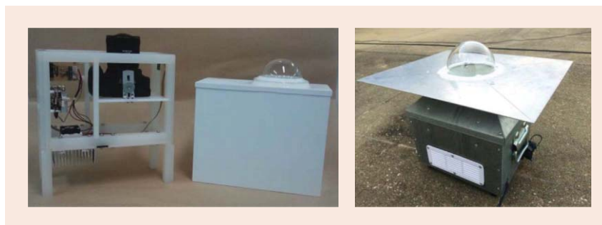
FIGURE 9. The design of the DIY Sky Imager.
