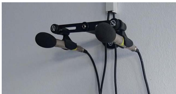
FIGURE 4. A microphone pair of the Localization of Acoustic Sources experiment that is attached to one of the walls of the Signal Processing Laboratory.
